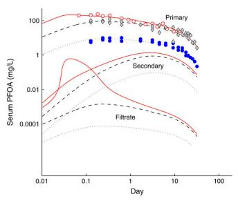
FIG. 6. Saturable resorption model predictions using parameters obtained with a maximum likelihood estimate show that the concentration in the filtrate compartment (dashed) spikes early on allowing the concentration in the primary compartment (solid) to rapidly converge for doses of 10 and 60 mg/kg.
